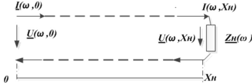
$$T_P(\omega, X_H) = T_u(\omega, X_H) \cdot T_i(\omega, X_H) = e^{-2 \cdot \alpha(\omega) \cdot X_H};$$
