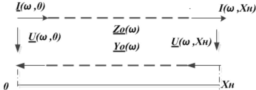
$$\underline{\gamma}_0^2(\omega) = \frac{\omega^2}{V_o^2} \cdot \frac{e^{j(\pi - \delta_\omega)}}{\cos(\delta_\omega)} = -\frac{\omega^2}{V_o^2} \cdot \frac{e^{-j\delta_\omega}}{\cos(\delta_\omega)};$$
