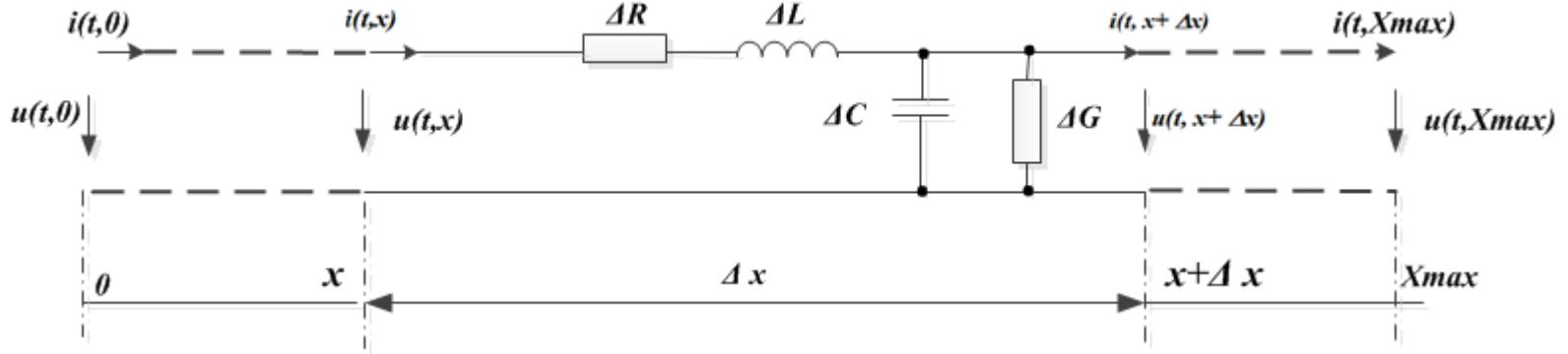
$$\begin{cases} \Delta \underline{U}(\omega, x) = \underline{U}(\omega, x) - \underline{U}(\omega, x + \Delta x) = \underline{Z}_0(\omega) \cdot \Delta x \cdot \underline{I}(\omega, x) \\ \Delta \underline{I}(\omega, x) = \underline{I}(\omega, x) - \underline{I}(\omega, x + \Delta x) = \underline{Y}_0(\omega) \cdot \Delta x \cdot \underline{U}(\omega, x + \Delta x) \end{cases}$$
