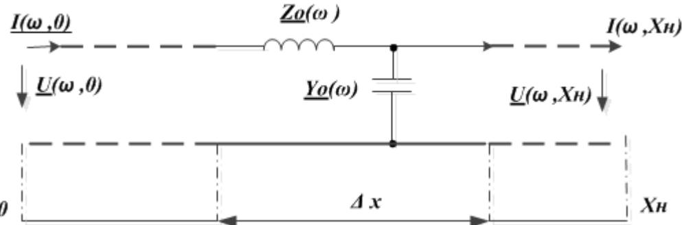
$$\begin{cases} \underline{U}(\omega,0) = \underline{U}(\omega,x) \cdot \cos\left[\frac{\omega}{V_w} \cdot x\right] + j \cdot Z_w \cdot \underline{I}(\omega,0) \cdot \sin\left[\frac{\omega}{V_w} \cdot x\right]; \\ \underline{I}(\omega,0) = \frac{j}{Z_w} \cdot \underline{U}(\omega,x) \cdot \sin\left[\frac{\omega}{V_w} \cdot x\right] + \underline{I}(\omega,x) \cdot \cos\left[\frac{\omega}{V_w} \cdot x\right]; \end{cases}$$
