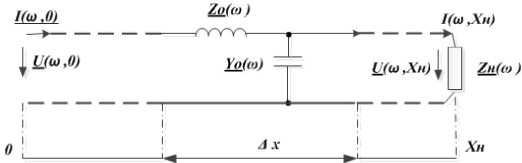
$$\underline{U}(\omega, X_H) = \left[ \cos\left(\frac{\omega}{V_w} \cdot X_H\right) - j \cdot \frac{Z_w}{Z_H(\omega)} \cdot \sin\left(\frac{\omega}{V_w} \cdot X_H\right) \right] \cdot \underline{U}(\omega, 0);$$
