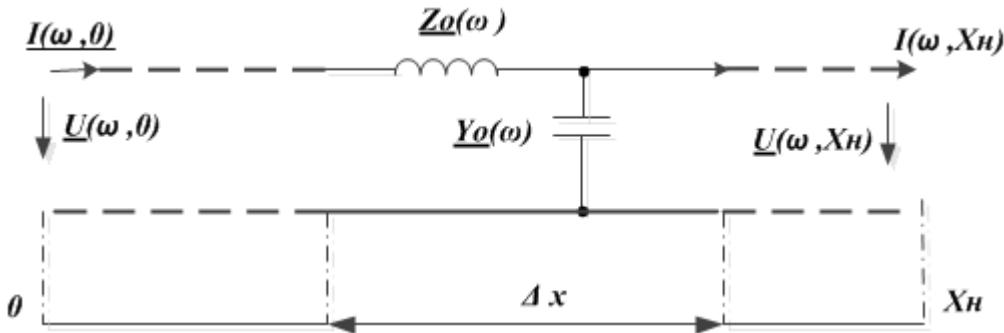
$$V_w = \frac{1}{\sqrt{L_0 \cdot C_0}}; \quad L_0 = \mu \cdot \lg\left(\frac{2 \cdot D}{d}\right); \quad C_0 = \frac{\varepsilon}{\lg\left(\frac{2 \cdot D}{d}\right)};$$
