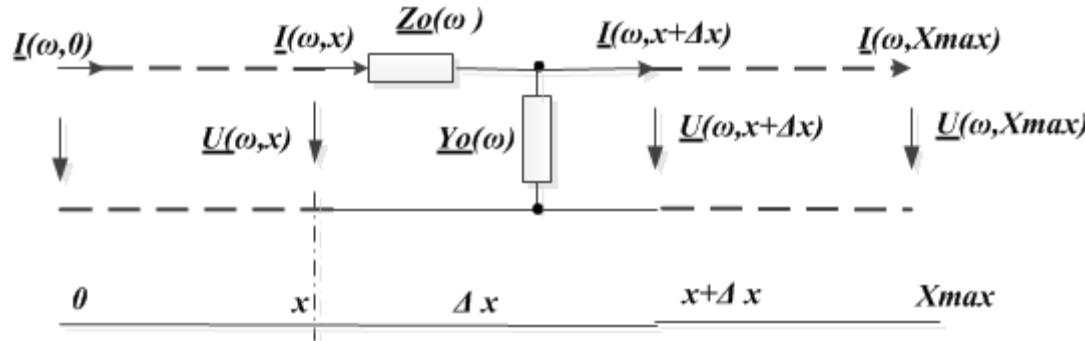
$$\underline{Z}_0(\omega) = [j \cdot \omega \cdot L_0 + R_0] \quad \left\langle \frac{O_m}{m} \right\rangle; \quad \underline{Y}_0(\omega) = [j \cdot \omega \cdot C_0 + G_0] \quad \left\langle \frac{C_m}{m} \right\rangle$$
