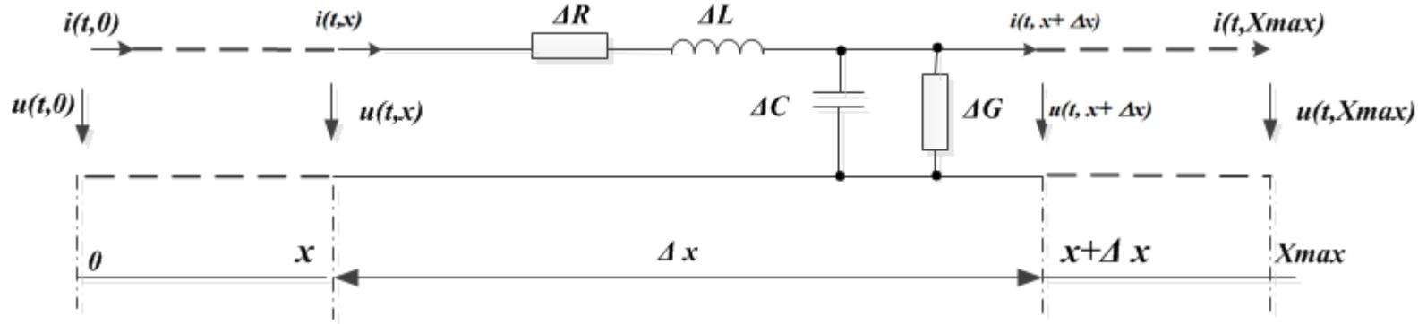
$$\underline{Z}_0(\omega) = [j \cdot \omega \cdot L_0 + R_0] \quad \left\langle \frac{O_M}{M} \right\rangle;$$
