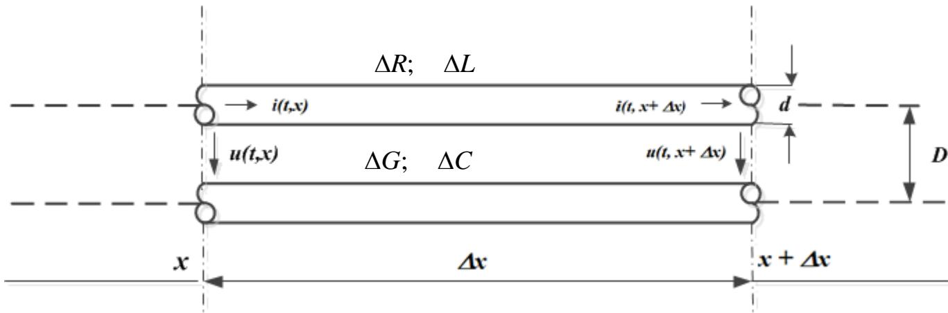
$$\Delta R = R_0 \cdot \Delta x; \quad \Delta L = L_0 \cdot \Delta x; \quad \Delta C = C_0 \cdot \Delta x; \quad \Delta G = G_0 \cdot \Delta x;$$
