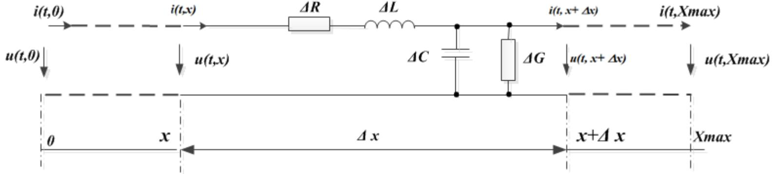
$$\begin{cases} \frac{\partial \underline{U}(\omega, x)}{\partial x} = -\underline{Z}_0(\omega) \cdot \underline{I}(\omega, x); \\ \frac{\partial \underline{I}(\omega, x)}{\partial x} = -\underline{Y}_0(\omega) \cdot \underline{U}(\omega, x); \\ \underline{U}_0 = \underline{U}(\omega, 0); \quad \underline{I}_0 = \underline{I}(\omega, 0); \end{cases}$$
