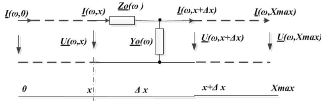
$$\underline{\gamma}_0(\omega) = \sqrt{\underline{Z}_0(\omega) \cdot \underline{Y}_0(\omega)}; \quad \left\langle \frac{1}{M} \right\rangle;$$
